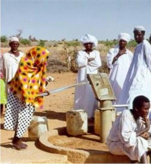
The India Mark III has similar configurations as the India Mark II, only the “down-hole components” were changed in order to improve the village level maintenance. The most important improvement is the “open top cylinder”, which makes it possible to remove the plunger and also the foot valve without lifting the cylinder and the entire rising main ( $\varnothing$  65 GI pipe). Cylinders are available in  $\varnothing$ 50 mm and  $\varnothing$ 62.5 mm.
