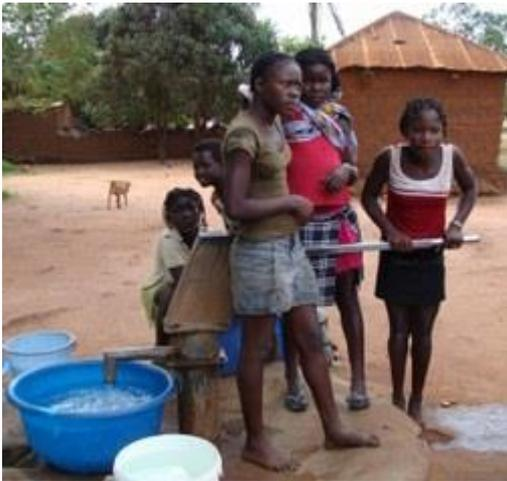
The India Mark II Pump is a robust conventional lever action handpump. It is designed for heavy-duty use, serving communities of 300 persons. The maximum recommended lift is 50 m.
